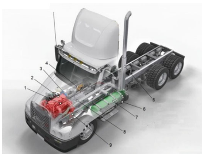
Fig. 44 Structure of a dedicated truck specially designed to work with LNG: 1—fuel injection system; 2—ICE; 3—electronic control module; 4—battery; 5—exhausting system; 6—fuel filter; 7—fuel container; 8—transmission; 9—fuel pipeline
