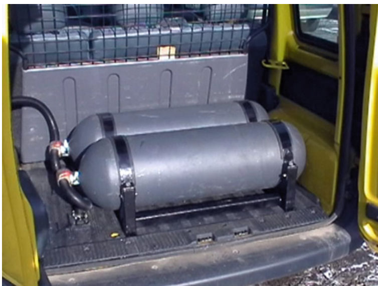
Fig. 9 Steel cylinders CNG, p_{\max} = 20 \text{ MPa}
