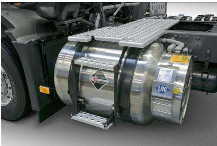
Fig. 10 Cryogenic LNG tank mounted in the truck [64]
