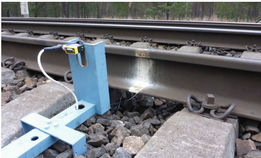
Fig. 21 Installation of optical diffuse sensor and accelerometer
