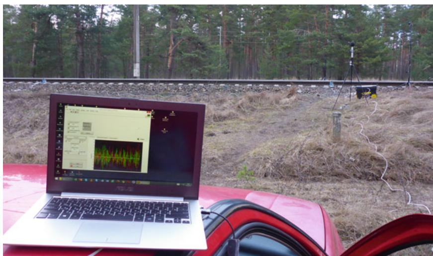
Fig. 24 Ethernet connection allows for remote PC location
