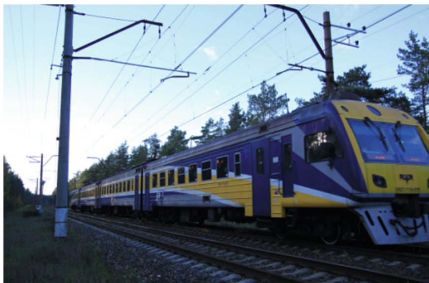
Fig. 4 The standard Latvian rail system. Track width—1520 mm, wheel diameter—920 1220 mm, conical wheels, differences in braking systems
