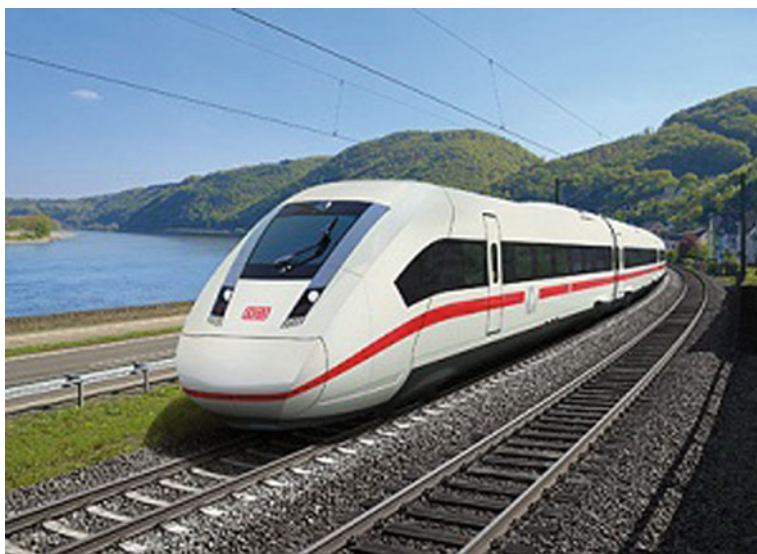
Fig. 3 The standard European rail system. Track width—1435 mm, wheel diameter—920 mm, cylindrical wheels
