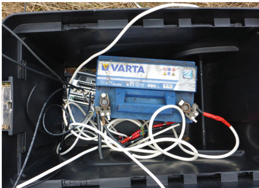
Fig. 23 NI data acquisition hardware and power source in a case
