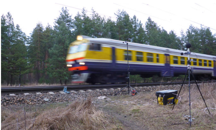
Fig. 22 Installation of measurement system in the field
